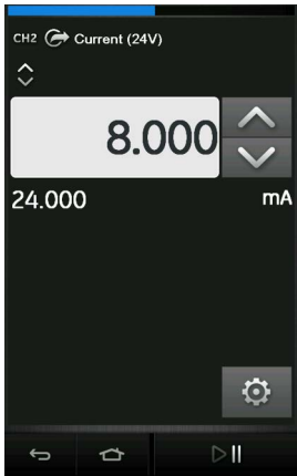
Figure 4-7: Source Current on CH2 with Internal Loop Power (Range: 0 to 24 mA)
