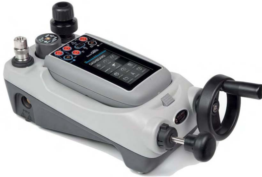
Figure 5-3: DPI 620 Genii with PV 62XG Pressure Station and PM 620 Pressure Module
