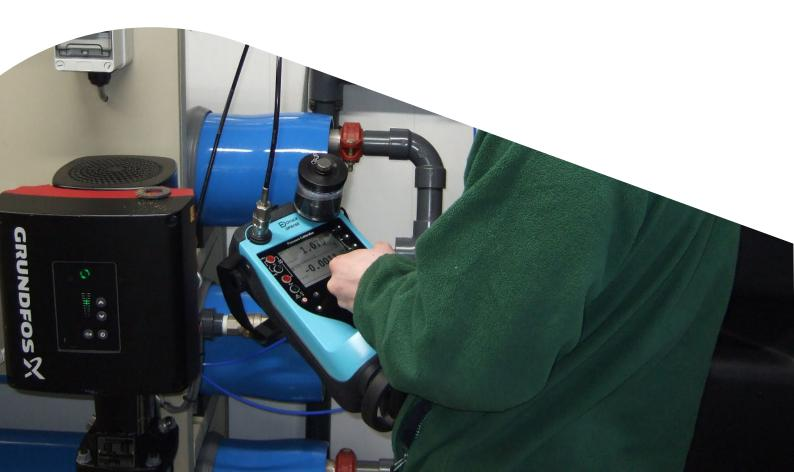
The DPI610E is an ultra-productive handheld pressure calibrator, built to perform across extreme environments. We are a global technology company that designs, develops and manufactures the highest quality, most accurate and reliable customized pressure sensing devices and instruments, software and services.
