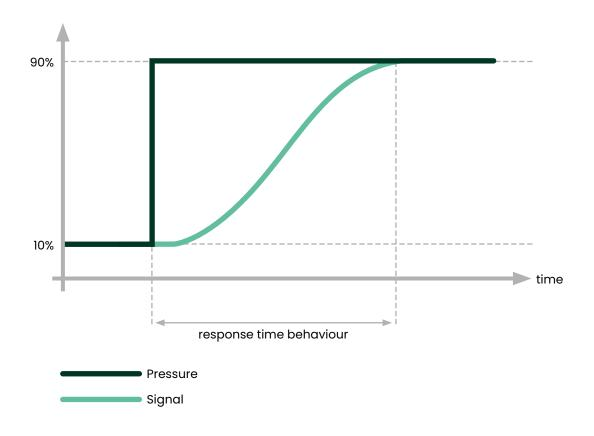
When taking readings at a speed approaching the response time it is possible to generate very large errors.
