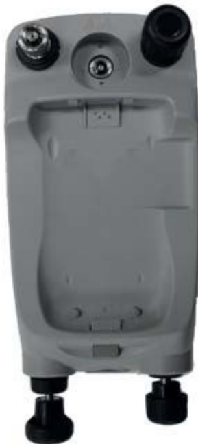
Safe area pressure station
