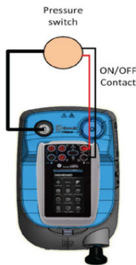
Figure 4-1: Switch testing setup
