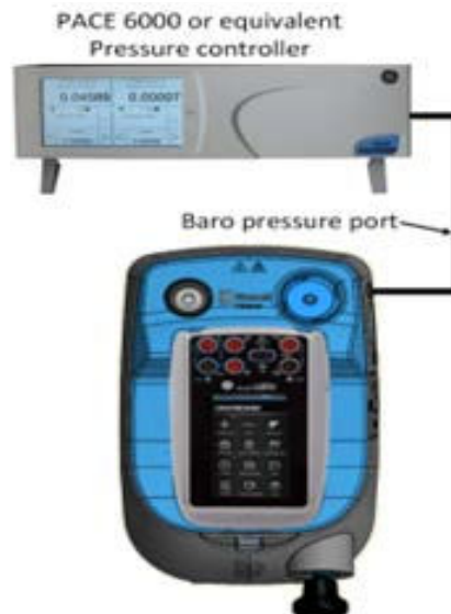
Figure 4-4: Barometer calibration setup
