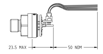
GAUGE SENSOR WITH PB PRESSURE CONNECTOR SHOW N
